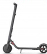
Ride Faster and Further Compared with 2019, the battery pack is now by Segway ES2 with 48V 13.5Ah battery, 150W motor and 25km/h max speed.
